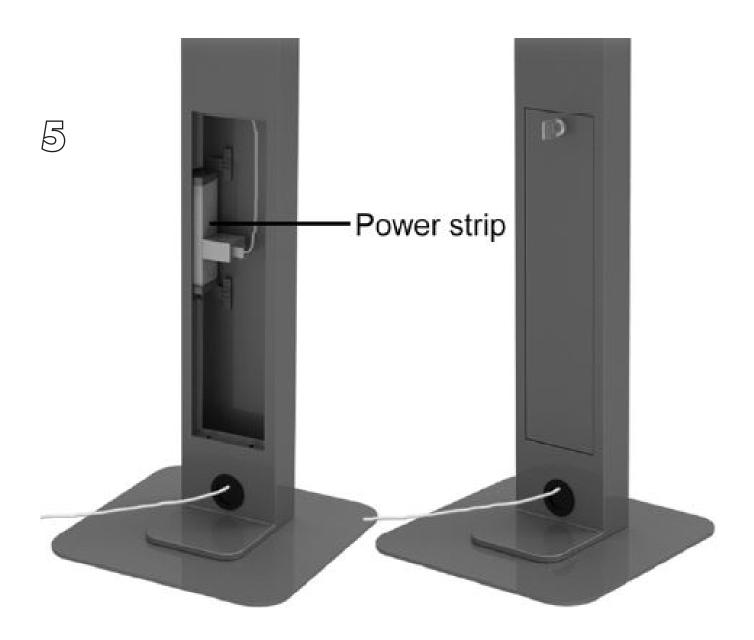
5. Open the door at the back of the stand. Plug the power adapter into the fixed power strip.6. Close and lock the door.
